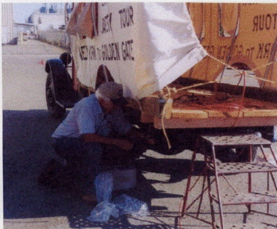
Al Garcia fitting bolts to the REO frame.
